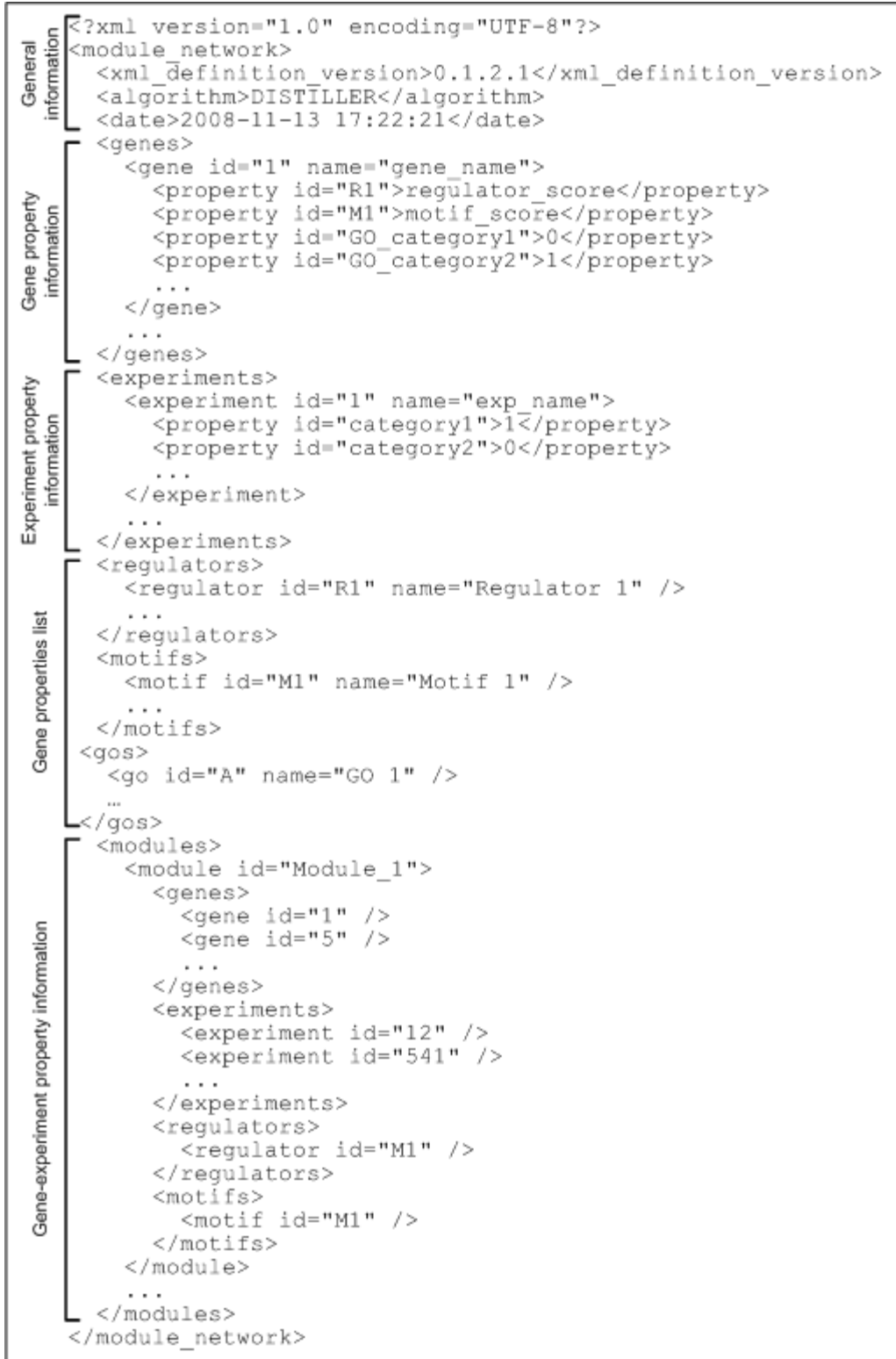
Figure 4: The structure of the module file. First some general information can be listed in the module file. Subsequently, the genes and possibly their properties are listed, followed by the experiments and their properties. Then the different gene properties such as the regulators or motifs are listed. Finally the actual module information is given. Modules minimally consist of genes and experiments, but also additional module properties like a regulator or motif are possible.
